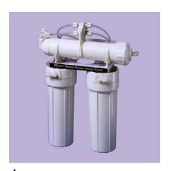
**SWT Premium™:** This 3 stage system features a 5 micron carbon block prefilter, 50 gpd TFC membrane, 4.5 gallon RO tank, and a 10 micron carbon block post-filter. Each unit includes a deluxe long reach faucet, angle stop adapter valve, water saving auto shut-off valve, and drain line check valve.
